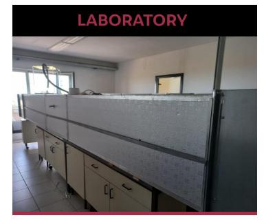
Following the requirements of the ISO 15714 regulation, an appropriate aeraulic duct has been created for testing and verifying the bactericidal and germicidal capacity of the UVC lamp.
