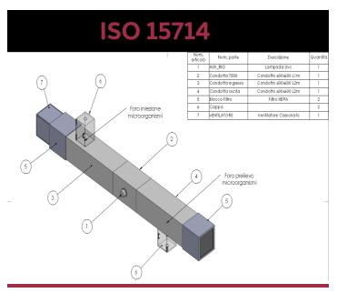
The UVC device has been tested following the regulation ISO 15714. The test was carried out by an ACCREDIA accredited laboratory. The experimental protocol was finally validated by the Department of Biology of the University of Bari Aldo Moro.
